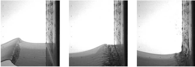
**Figure 8** – Breaking of the leading wave induced by wave type A at large scale
