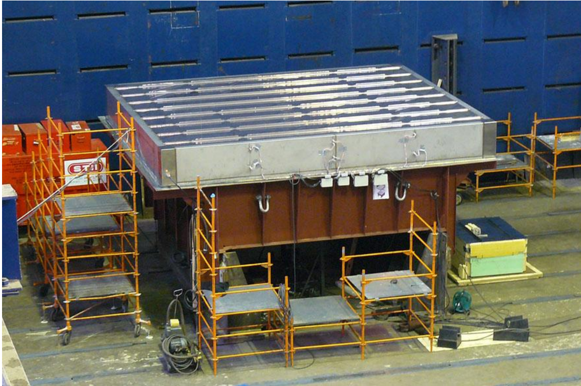
Fig. 11: General view of side grillage mock-up on test bench
