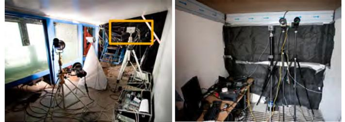
Figure 3. Location of high speed cameras at large (left) and full (right) scales
