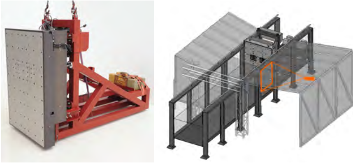
FIGURE 4: Test set-up at large scale. Rigid test wall alone (left) and installed in the flume (right).
