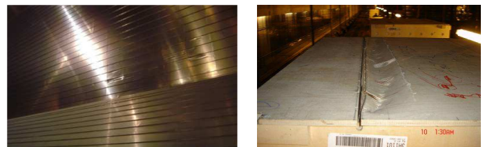
Figure 10: indented primary membrane (left) and deflected top cover (right)
