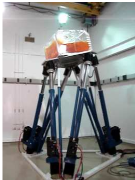
Figure 8: 6 d.o.f. test rig
