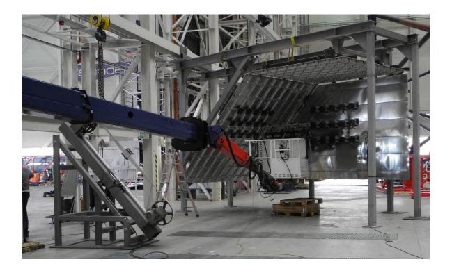
The immobilization system has been tested by clamping the basket on the mock up tank membrane wall, then upper chamfer, then ceiling in spite of its movements (before clamping). After clamping, every movements between basket and membrane was suppressed, despite of alternative load applied on telescopic arm simulating the tank's movement on which telescopic arm base is fixed.
