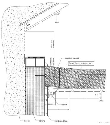
Thanks to this device, in case of displacement of the structure led by a seismic event, this one will enter into contact with the containment system with a limited force. The energy resulting from this displacement is absorbed by this shock absorber. The system is installed all around the periphery of the structure and is sized according the energy which has to be dissipated. Installed just above the liquid level, the material shall be able to ensure its function in cryogenic condition.
