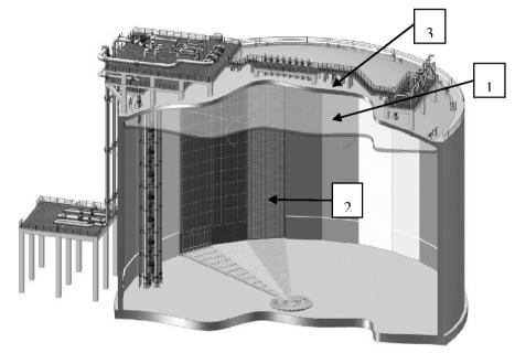
For geographic areas where the geotechnical data lead a significant movement of the suspended ceiling during a seismic event, the conventional designs imply the installation of a specific reinforcement on the structure periphery. This reinforcement is made of a beams network used to stiffen the structure and limit its displacements. The objective is to avoid a violent impact between the rigid structure and the metallic membrane with a risk of damaging the integrity of the primary membrane.
