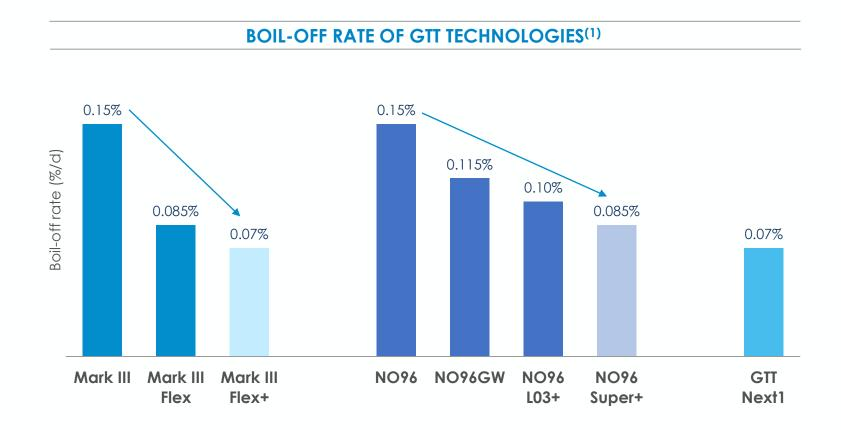
Enabling better energy efficiency by halving boil-off rate in a decade
