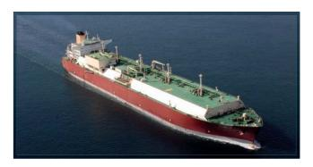
Seven large-capacity ethane carriers are already in service, using the technologies developed by GTT. In 2020, GTT received an order to design the tanks for four new ethane carriers. These latest-generation ethane carriers will be the largest ever built in the world (98,000 m³). This latest order is testament to the viability of GTT's containment systems for the transportation of various types of liquefied gas (other than LNG).
