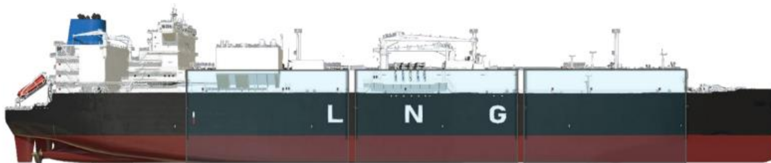
Three identical cargo tanks (same length)
