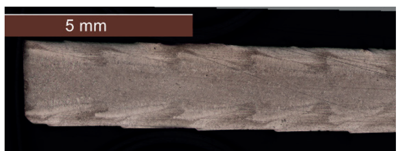
Figure 9: Longitudinal macro-examination of seam welding with the new inverter
