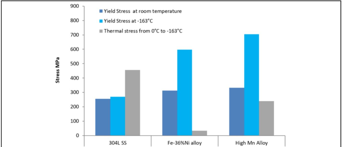
Figure 2: Mechanical and thermal properties of our high-manganese alloy compared to 304L stainless steel and Fe-36%Ni alloy
