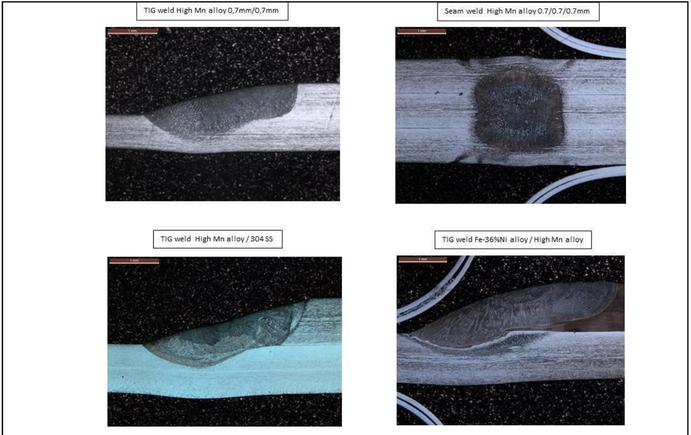
Figure 3: Illustration of welded samples with High Manganese Alloy
