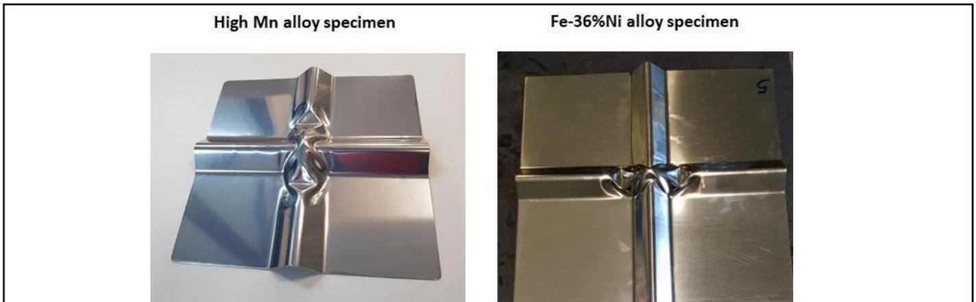
Figure 5: High Manganese alloy and Fe-36%Ni alloy corrugated specimens
