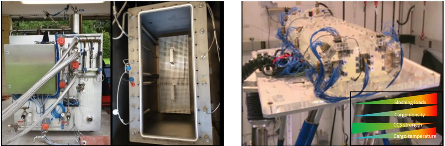
Figure 2: The technical developments to achieve multigas compliance includes material compatibility immersion tests and detailed analysis on CCS strengths under different cargo densities and temperatures.
