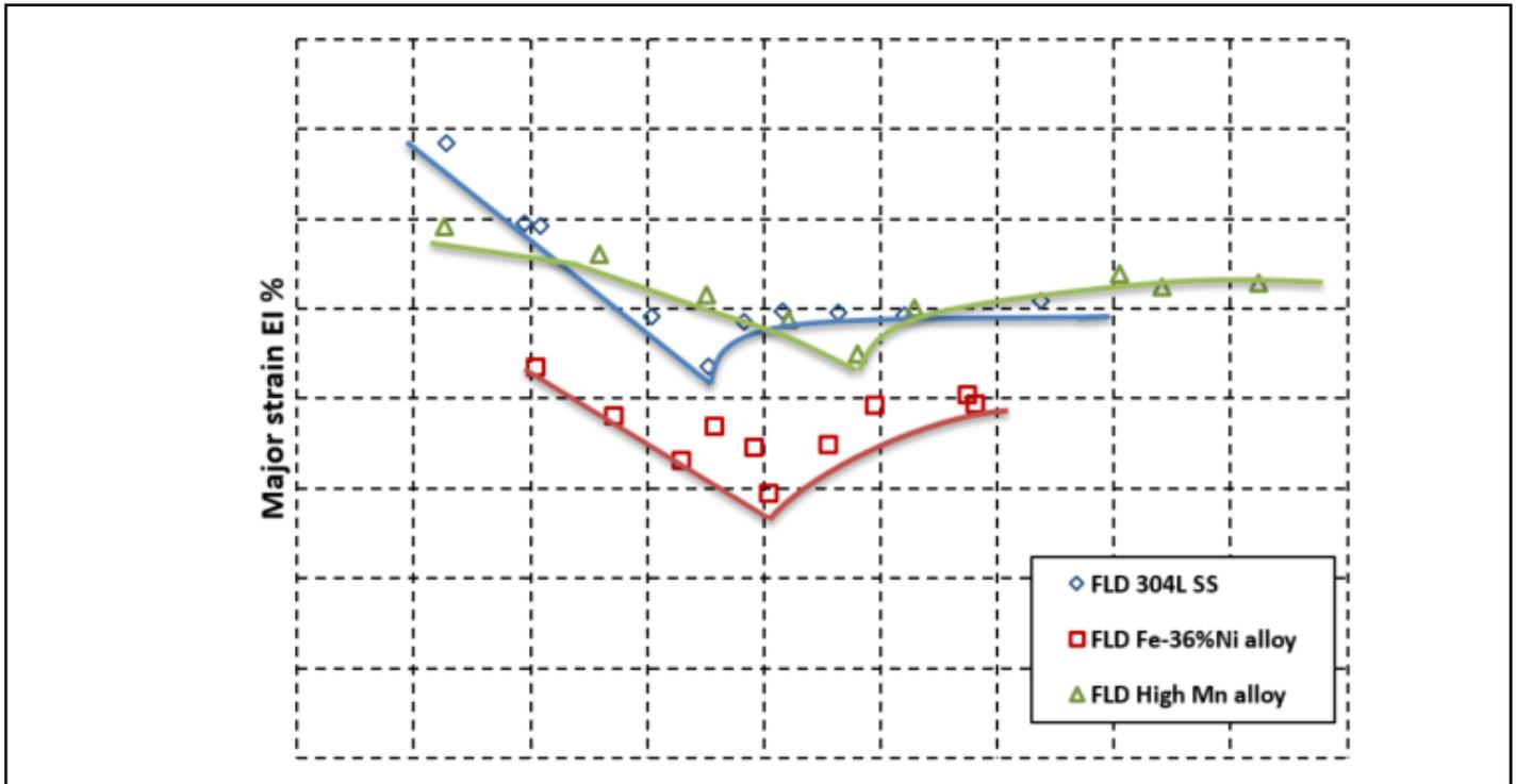
Figure 4: Forming limit diagram
