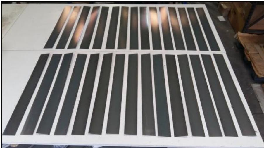
Figure 1: High Manganese 1mm thick sheets – semi-industrial trial
