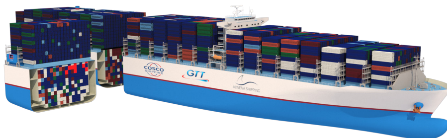
LNG retrofit and Jumboisation applied to a 14,000TEU container vessel
