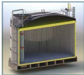
GTT received several orders for onshore storage tanks in 2020. The first one, received in June 2020 from Beijing Gas Group (BGG), relates to the design of two full integrity LNG membrane storage tanks as part of the BGG Tianjin Nangang LNG terminal. These two tanks with a capacity of 220,000 m<sup>3</sup> each should be commissioned at the end of 2022 and will be the largest onshore storage tanks in China.
