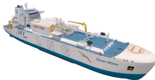
“Ballast-Water-Free” LNG Bunker & Feeder vessel design
