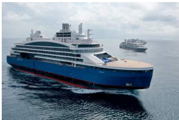
Figure 2. Le Commandant Charcot , the very first polar cruise vessel using LNG as fuel, fitted with two membrane fuel tanks (total capacity of 4500 m 3 ) designed to 2 bar gauge. Image courtesy of Ponant.
