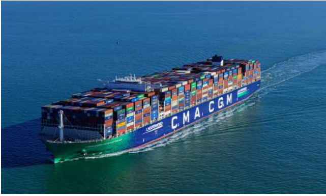
Figure 3. CMA CGM JACQUES SAADE, the first 23 000 TEU containership fuelled by LNG fitted with one 18 600 m 3 Mark III membrane fuel tank. Image courtesy of CMA CGM.
