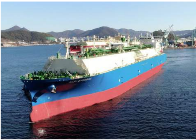
Figure 4. SERI EVEREST the world's largest VLEC (98 156 m 3 ) to be granted ABS notation 'LNG Cargo Ready' contributing to ethane market development and opening perspectives for ultra large ethane carrier designs. Image courtesy of MISC.
