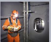
The TAMI test was introduced by GTT in 2011 as an alternative method of assessing the integrity of the secondary barrier on membrane containment systems. The TAMI test can be carried out inservice or at quay side,
