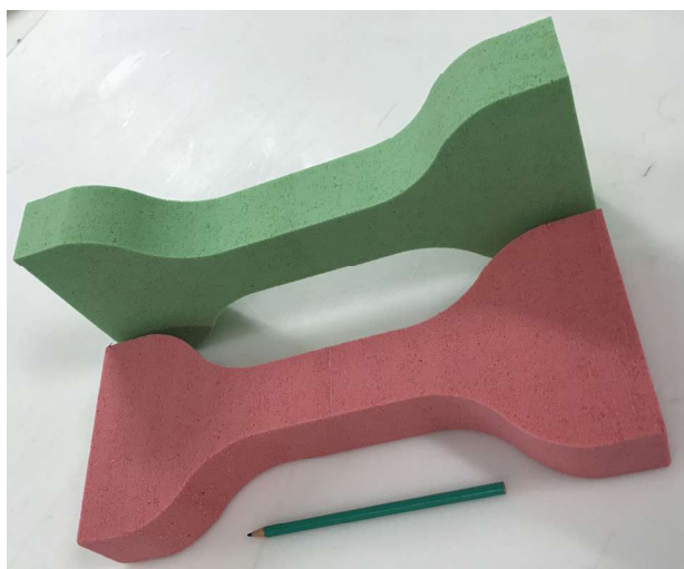
Figure 2. Tensile test specimen for cellular materials.
