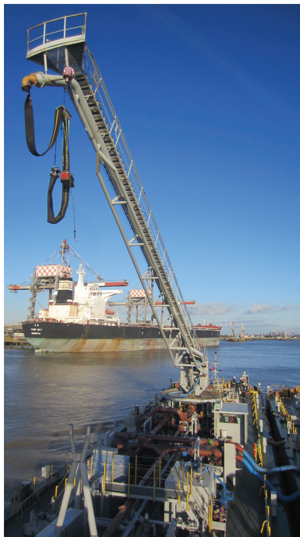
Figure 3. Existing bunker mast for conventional fuel.
