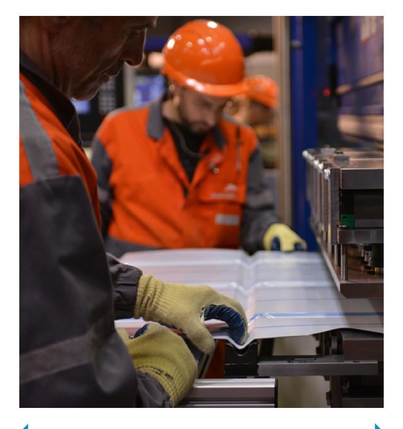
The Mark III LNG tank technology uses 3-m-by-1-m sheets of corrugated stainless steel that are welded into place to form the primary tank membrane.
