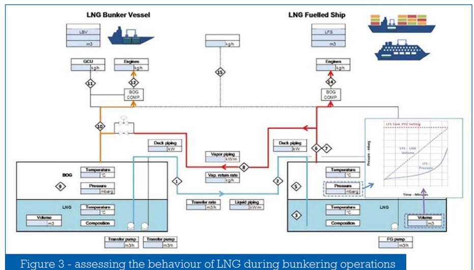
Figure 3 - assessing the behaviour of LNG during bunkering operations
